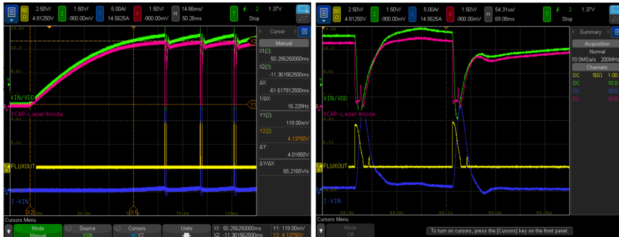
Figure 27: Laser firing GaNFET Short Circuit Protection engaged when V_{IN} & V_{DD} are biased from the same supply and zoom in view (cathode sense)
